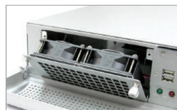
Front Replaceable Air Filters/Fans
